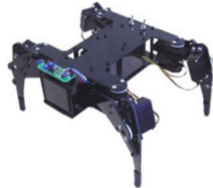
Fig. 6.1 ANIBOT. To the best of our knowledge, this is the first quadruped robot controlled by a CPG electronic circuit built based on the 8-network proposed by Golubitsky et al. [61, 62, 146, 148]
